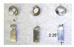
Arc-melted and drop-casted ingots
