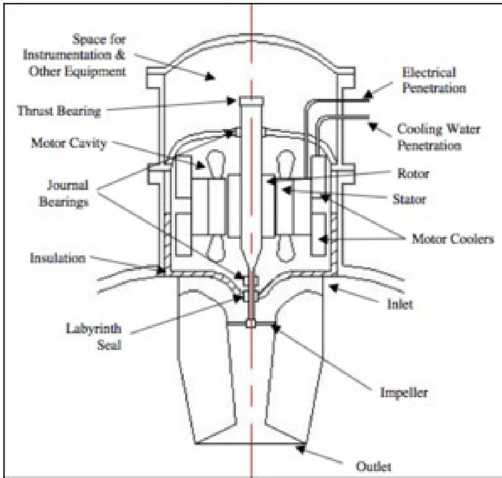
Figure 1-6. Simplified Sketch of a Typical Submerged Gas Circulator Layout
