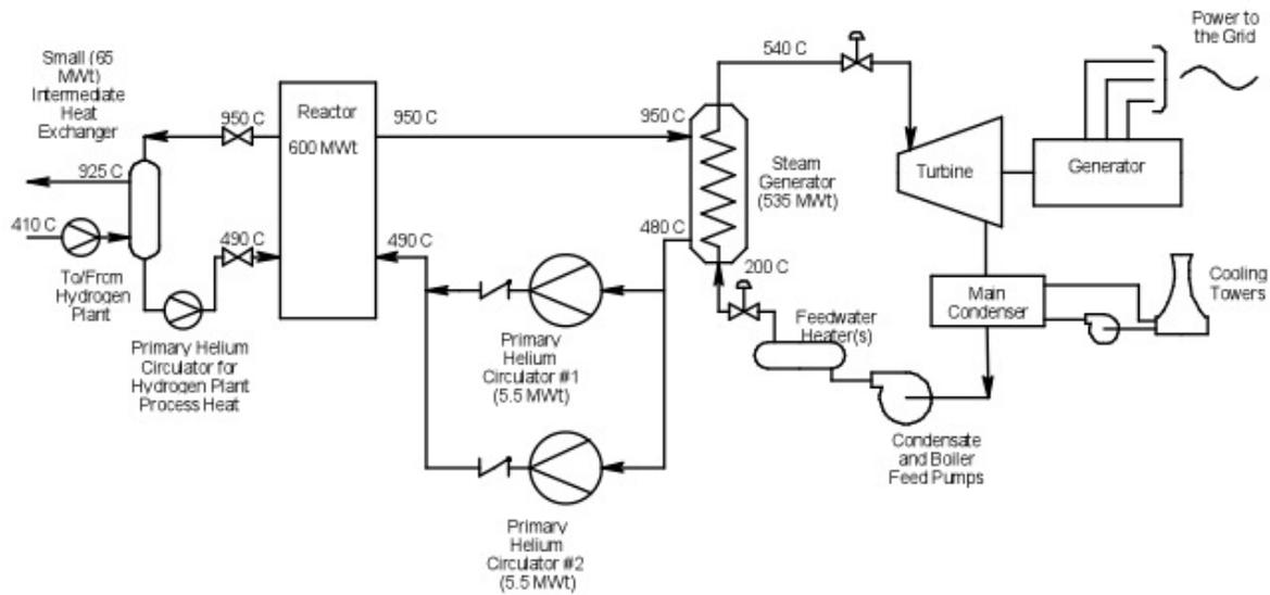
Figure 1-2. NGNP Configuration with Two Parallel Main Helium Circulators
