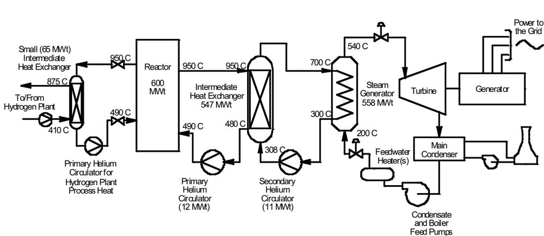
Figure 1-3. NGNP Indirect Cycle Configuration
