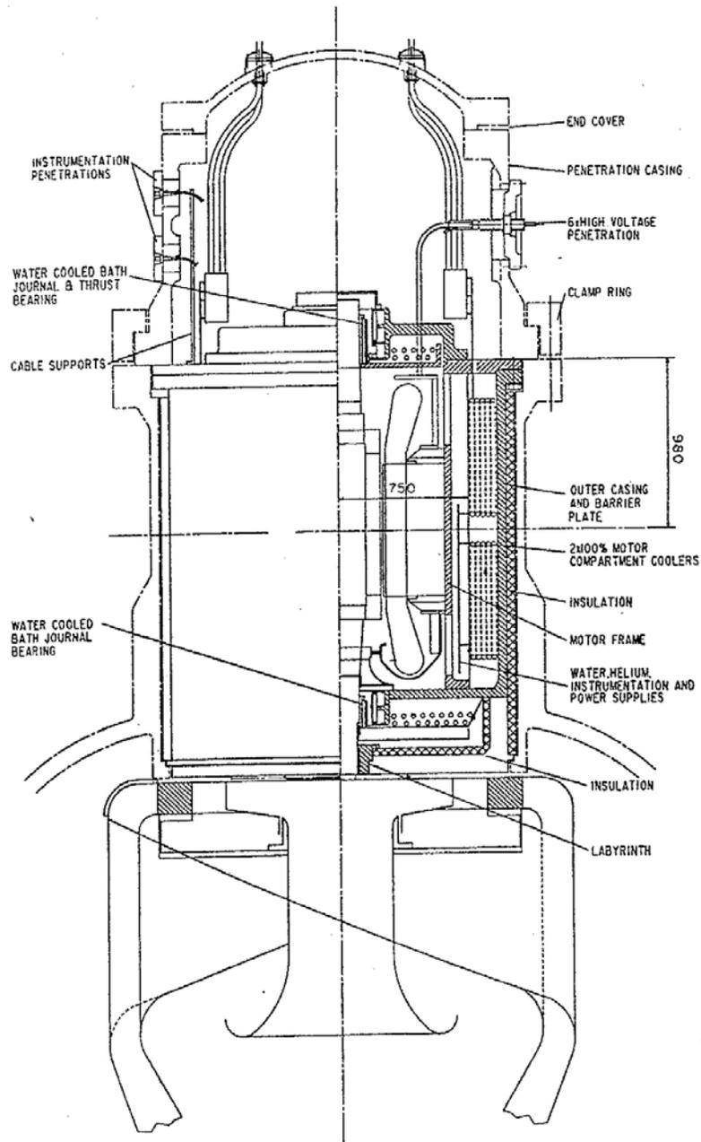
Figure 1-4. General Atomics MHTGR NPR Helium Circulator Drawing
