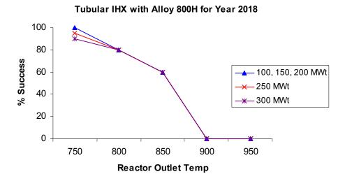
Figure 5. Year 2018 Percentage Success for the Tubular IHX manufactured from Alloy 800H
