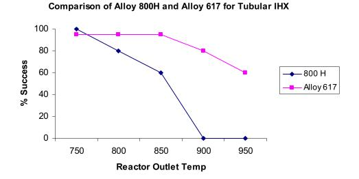
Figure 6. Comparison of % success for Tubular IHX with Alloy 617 vs. Alloy 800H at 100 MWt
