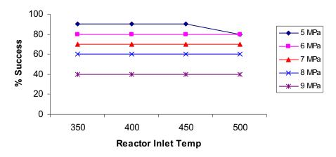
Figure 20. Year 2018 percentage success for Vessel System with 2.25Cr1Mo at 250 MWt
