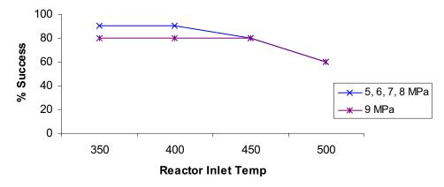
Figure 18. Year 2018 percentage success for Vessel System, cooled SA-508 at 250, 350 MWt
