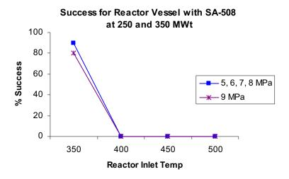
Figure 16. Year 2018 percentage success for Vessel System with SA-508 at 250 and 350 MWt
