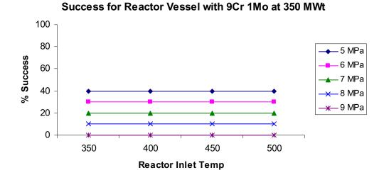
Figure 14. Year 2018 percentage success for Vessel System with mod 9Cr1Mo at 350 MWt
