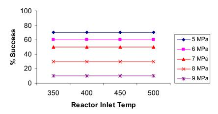
Figure 22. Year 2018 percentage success for Vessel System with 2.25Cr1Mo at 550, 650 MWt
