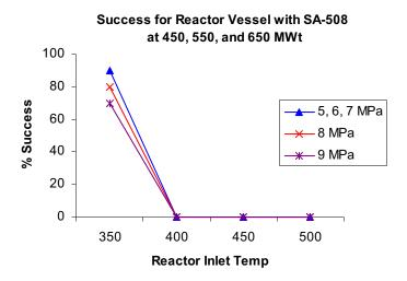
Figure 17. Year 2018 percentage success for Vessel System with SA-508 at 450, 550, and 650 MWt
