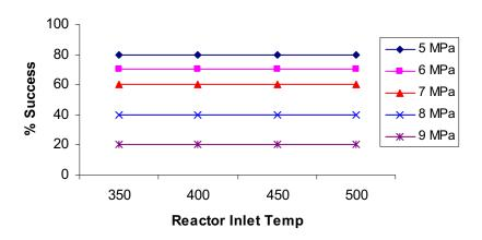
Figure 21. Year 2018 percentage success for Vessel System with 2.25Cr1Mo at 350, 450 MWt
