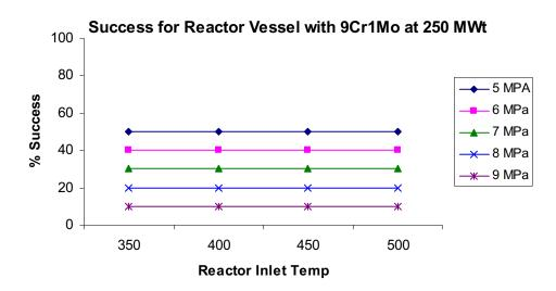
Figure 13. Year 2018 percentage success for Vessel System with mod 9Cr1Mo at 250 MWt
